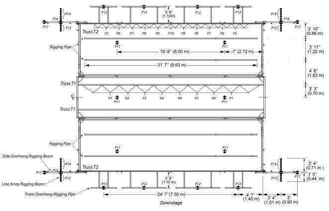
**MAXIMUM ROOF LIFTING CAPACITY: 12000 LB (5443 KG)**
